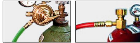
Attach hoses. Green hose to oxygen (right hand thread). Red hose to gasoline (left hand thread).
