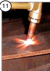
Warm the tip by pressing it to steel at an angle. Adjust gas valve until the steel turns a bright red orange.
