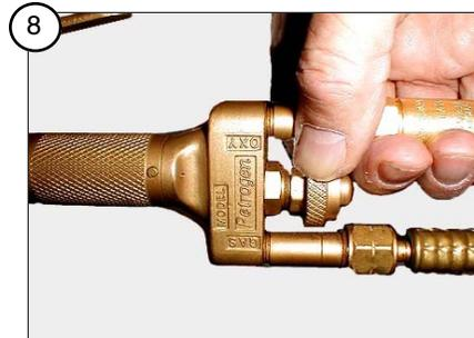
Then open torch gasoline valve until light mist appears. If liquid drips from torch, increase oxygen or reduce gasoline.
