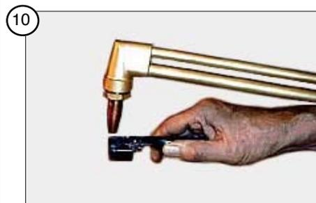
Ignite torch by striking spark close to the tip and to one side. A new hose contains air which extinguishes the flame. Just light again - about 2 or 3 times until line is purged of air.
