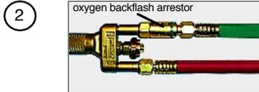
Install oxygen backflash arrestor between torch and oxygen hose. No need for a fuel line backflash arrestor.
