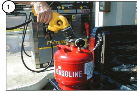
Fill tank only at a gasoline station. Gasoline must be fresh (not over 4 months old) and not contaminated with oil or diesel fuel. Low-octane fuel works fine.
