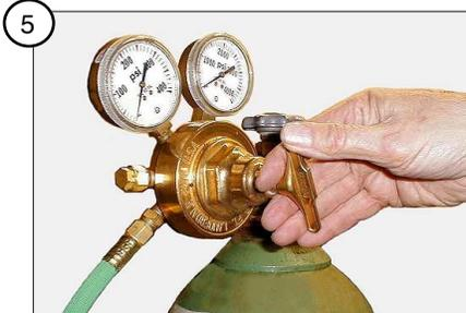
Select cutting tip and oxygen pressure from cutting chart on gasoline tank. Open oxygen bottle valve slowly and fully. Set desired pressure on oxygen regulator.
