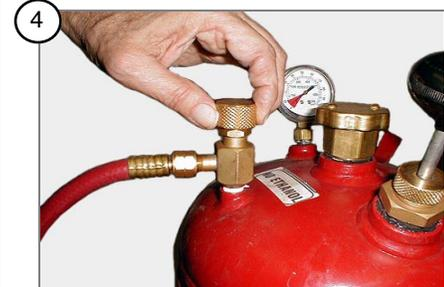
Open tank gasoline valve slowly, about 2 turns. After 30 seconds, open valve fully. If gasoline is shut off by fast flow valve, close valve, tap tank on the ground and repeat.
