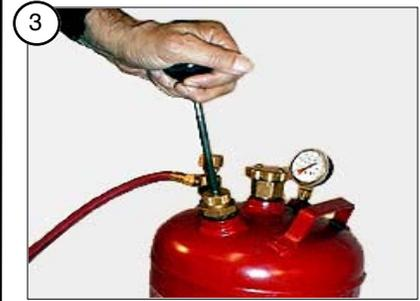
Pump tank to 20 psi. Pressure drops as torch cuts. When it drops to 10 psi, pump back to 20 psi.
