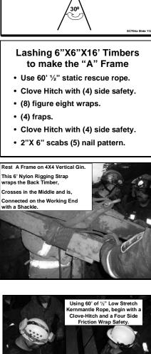
Carry the Timber "A" Frame and Perform a "Flat Ladder Raise" while Footing the Legs.
